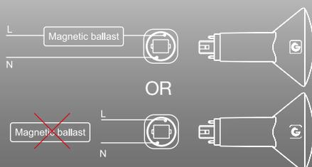
When used with a magnetic ballast, the PL V can function as a plug & play lamp and operate with the existing ballast. If the ballast is not compatible, it can be bypassed and the lamp can run directly off line voltage.
